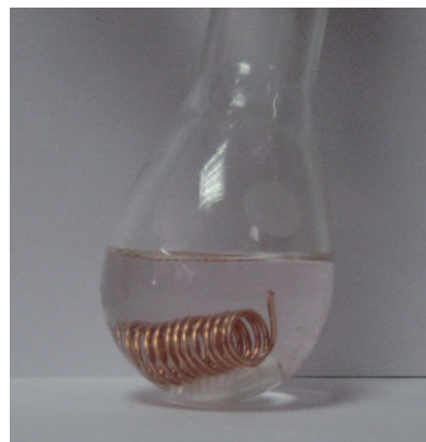
Figure 1. A photograph of the ARGET ATRP reaction of MMA with CDB and a copper wire as the reducing agent. Flask contents: [\text{MMA}]_0/[\text{CDB}]_0/[\text{CuBr}]_0/[\text{TPMA}]_0 = 30,000:1:0.01:0.03 ; MMA/anisole = 1:1 (v/v); copper(0) wire l = 30 \text{ cm} , d = 1 \text{ mm} .
